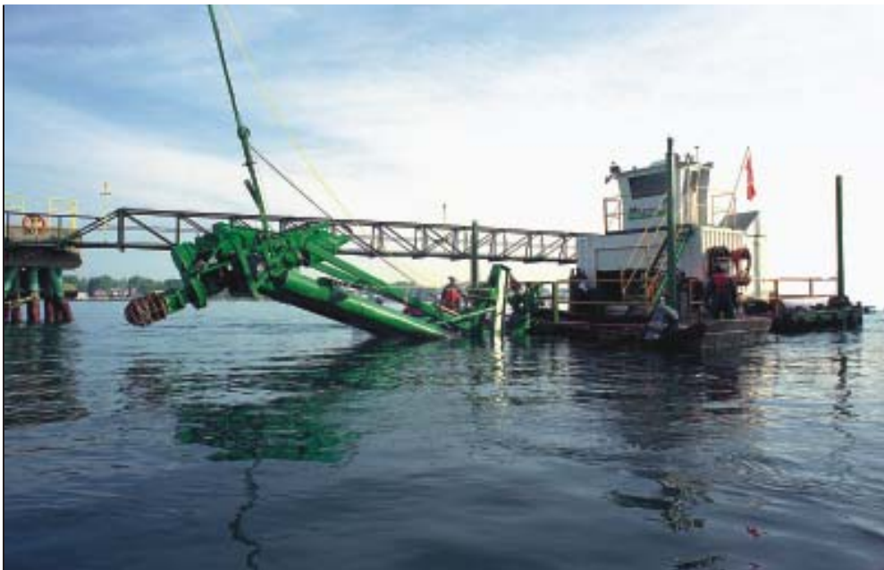
In Spring 2002, Dow Canada's Sarnia (Ontario) Site began a multi-phase program using the latest in hydraulic dredging technology (unit pictured) to remove historically contaminated sediment from the bottom of the St. Clair River adjacent to the company's site.
